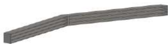
Fig. 1 Design of miter gate-inspired beam of 2mm thickness, 2 ribs, and 15° mating angle
