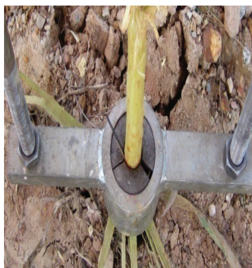
FIGURE 1. Root gripping by wedge and barrel
