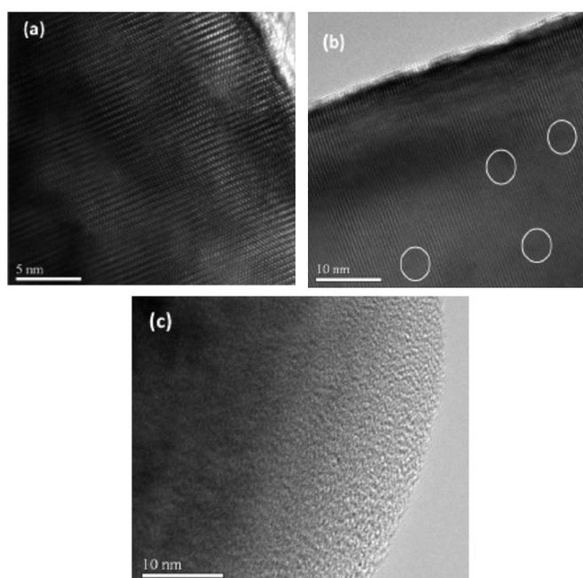
FIGURE 1. HRTEM images of the a) un-irradiated ZnO NWS b) C irradiated at the dose of  $1 \times 10^{13}$  ions/cm<sup>2</sup> and c) C irradiated at the dose of  $1 \times 10^{15}$  ions/cm<sup>2</sup>
