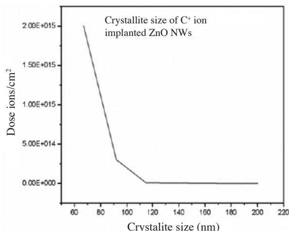
FIGURE 3. Crystallite sizes of C<sup>+</sup> ion implanted ZnO NWs
