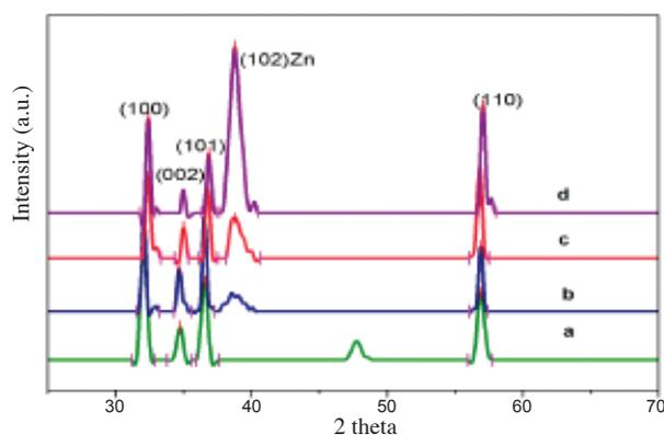
FIGURE 2. XRD patterns of carbon ion irradiated ZnO nanowires a) Un-irradiated ZnO nanowires, b)  $1 \times 10^{12}$  ions cm<sup>-2</sup>, c)  $1 \times 10^{13}$  ions cm<sup>-2</sup> and d)  $1 \times 10^{14}$  ions cm<sup>-2</sup>
