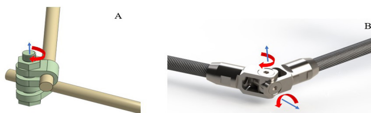
FIGURE 6. A. Type 1 external fixator connector rod with one DOF. B. Newly designed type 2 connector rod with a universal joint and two DOFs
