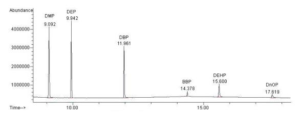
Figure 1: The total ion chromatogram of six phthalates at the concentration of 25 mg/L obtained by full-scan mode (TIC).
