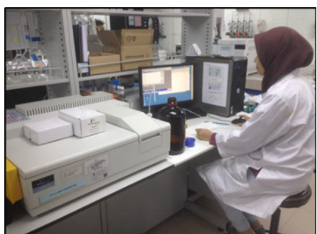
FIGURE 5. The student is analyzing samples using UV-Vis Spectrophotometer
