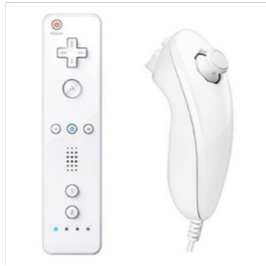
FIGURE 2. Wii controller with an accelerometer and Motion Plus expansion device (Steven 2012).
