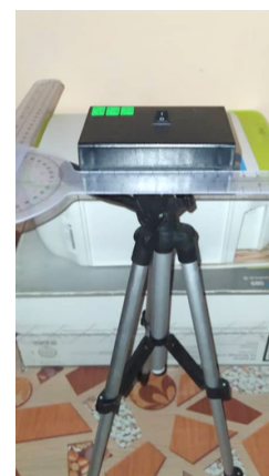
FIGURE 10. Setup for measuring the accuracy of the MPU6050 Sensor by using a Goniometer tool.
