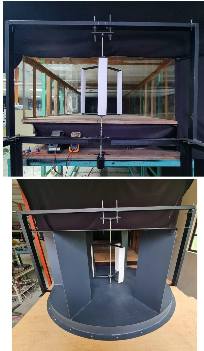
FIGURE 7.(a) open Darrieus VAWT (without GWs) (b) Darrieus VAWT (with GWs)
