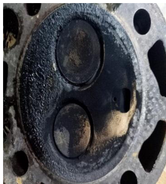
FIGURE.3 Macroscopic view of engine head deposit operated with DF95WC05.
