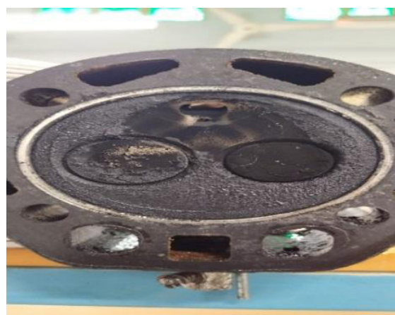
FIGURE.2 Macroscopic view of engine head deposit operated with DF
