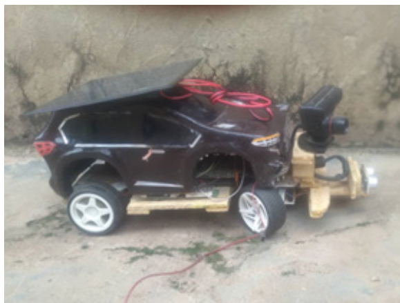
FIGURE 8. Fully assembled solar-powered autonomous vehicle
