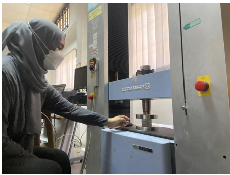
FIGURE 3. Compressive strength test of cube
