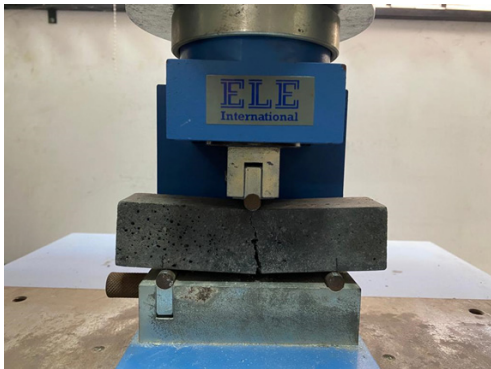
FIGURE 4. Flexural strength test of the prism
