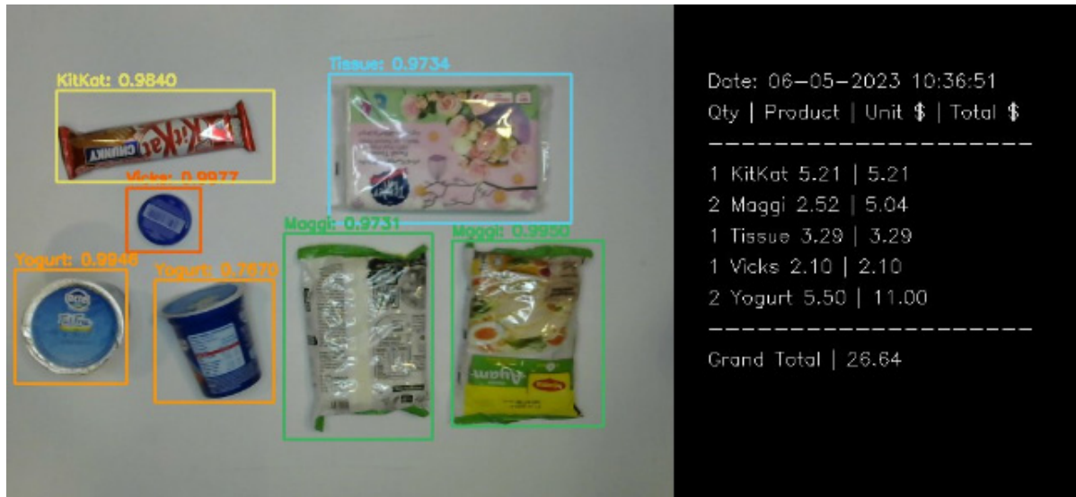
FIGURE 5. A transaction notification showing the augmented image of the checked out items, affixed with corresponding itemized bill. Upon transaction approval by the customer, this record is sent to the system administrator via the Telegram instant messaging platform
