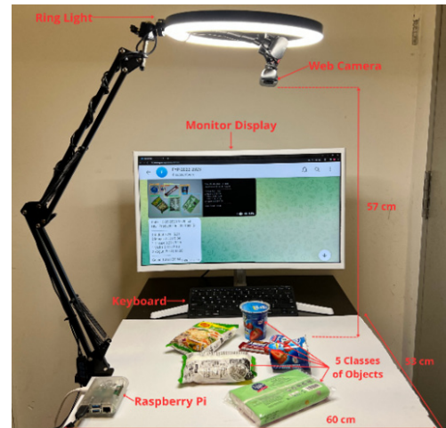
FIGURE 2. The system setup for implementing the trained model, with a sample of checkout items placed on the countertop under the web camera
