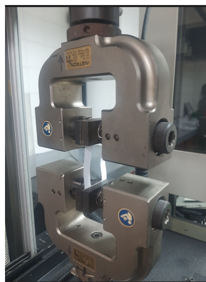
FIGURE 2. Sample arrangement for tensile test
