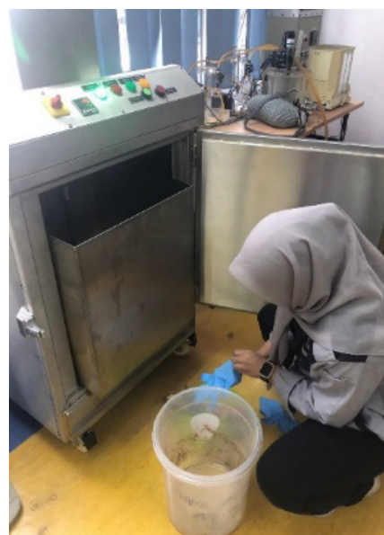
FIGURE 2. Machine to heat and dry the food waste
