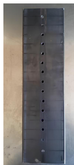
FIGURE 3. Typical pre-drilled intermittent weld holes
