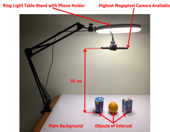
FIGURE 1. The photography setup used to capture 200 dataset images of common food items in Malaysian households
