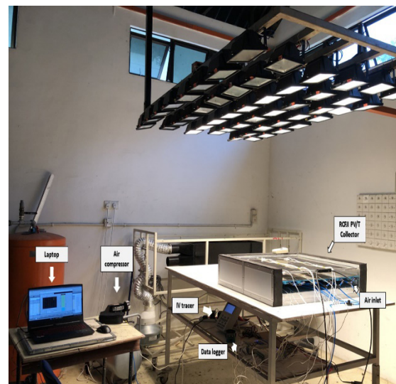
FIGURE. 3 In-house experiment setup using a solar simulator
