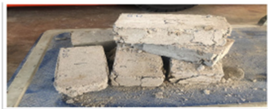
FIGURE 6. Failure mode of bricks specimen
