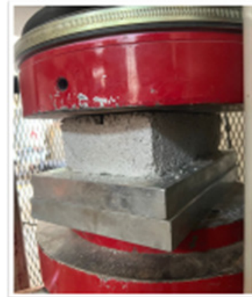
FIGURE 4. Compressive strength test
