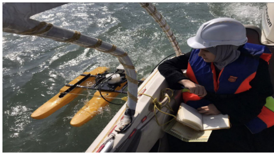
FIGURE 3. Measurement of bed levels, water depths and velocities using the M9 device
