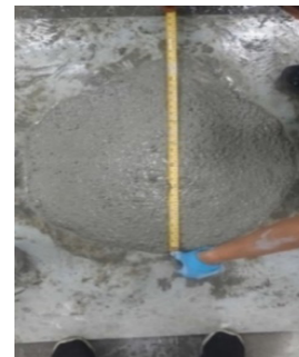
FIGURE 1. Slump flow test
