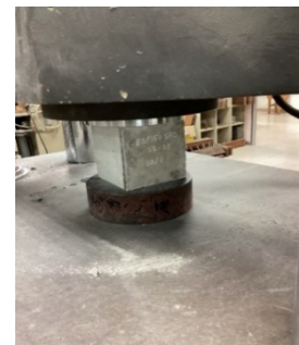
FIGURE 3. Experimental set-up of SCC under compressive loading
