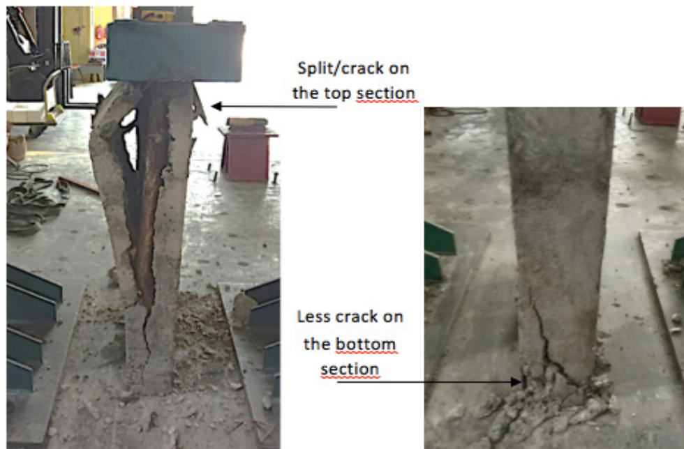
(a) Top failure
