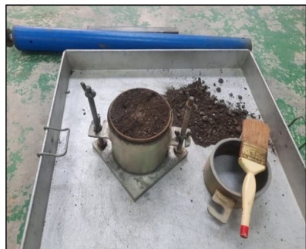
FIGURE 3. Modified proctor test specimen
