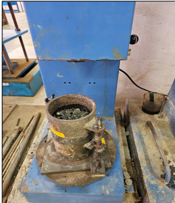
FIGURE 4. Bulk density specimen
