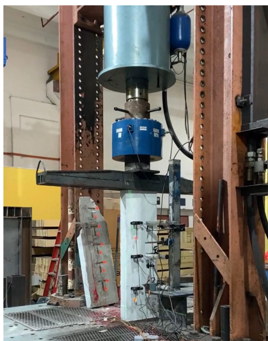
FIGURE 2. Compression test using reaction frame machine.
