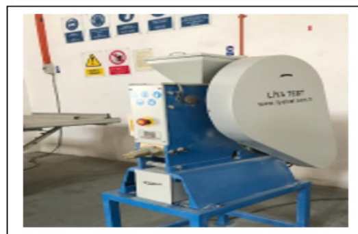
FIGURE 1. a) Collection of the tested cubes b) Jaw crusher was used for crushing the tested cubes.
