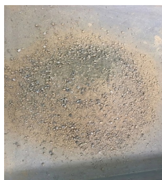
FIGURE 2. Recycled Concrete Aggregate passing 5 mm sieve.
