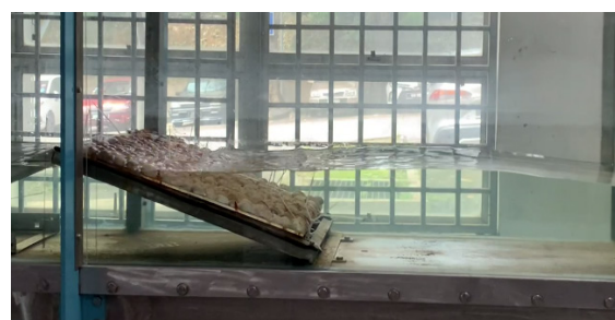
FIGURE 24. Shot reveal demonstrates the wave structure on the regular wave emerged condition. ( T=0.10s ).
