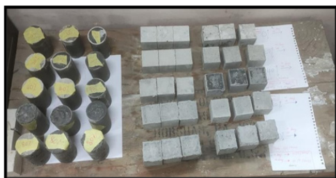
FIGURE 1. Concrete specimens of different mixes
