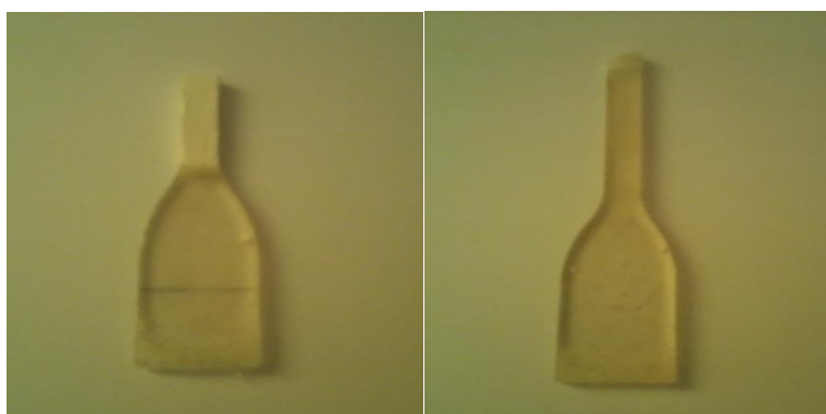
Figure 5. Visualization of deformed samples under tensile test
